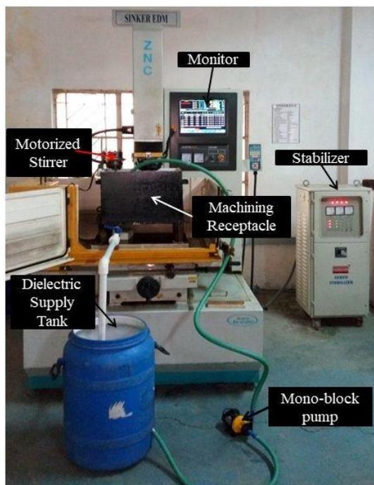
Fig. 1. PMEDSP Set-up
