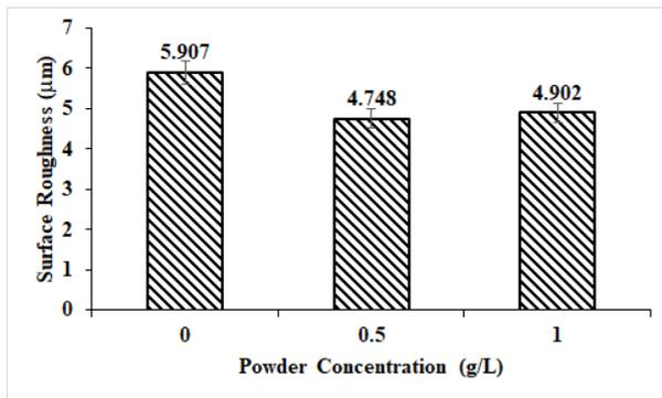
Fig. 3. Variation of surface roughness with powder concentration
