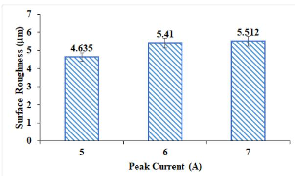
Fig. 4. Variation of surface roughness versus peak current
