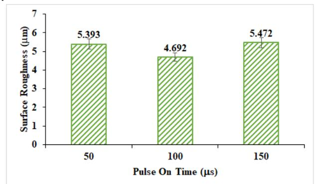
Fig. 5. Variation of surface roughness versus pulse-on time
