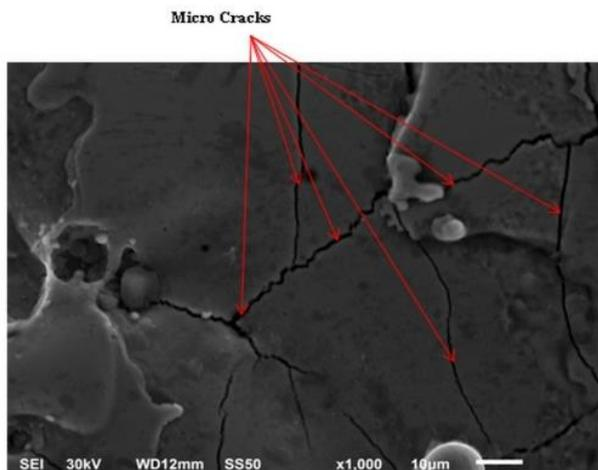
Fig. 7. Micro-cracks on the surface machined with unblended dielectric
