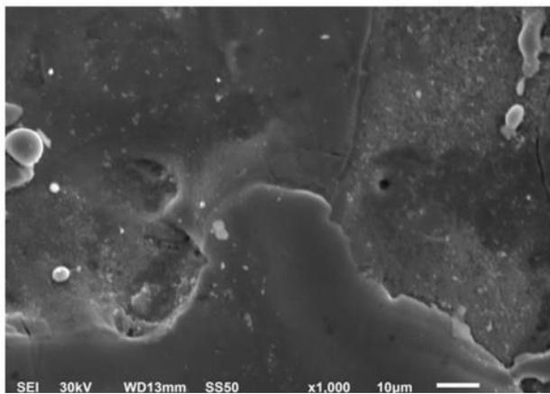
Fig. 8. Micro-cracks on the surface machined with blended dielectric
