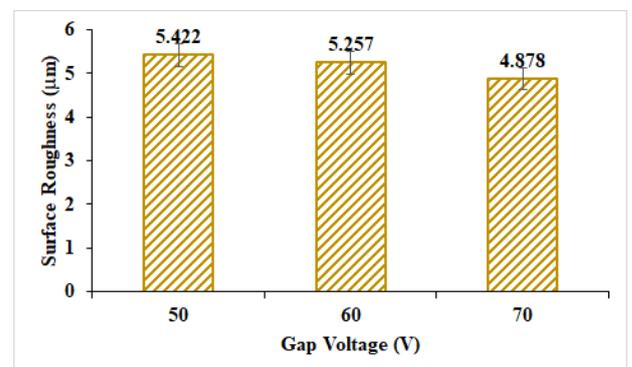
Fig. 6. Variation of surface roughness with gap voltage
