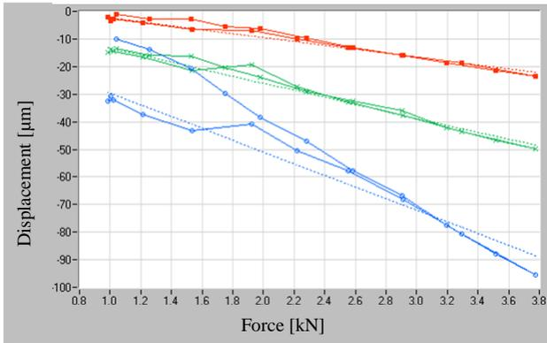
Fig. 8. Stiffness characteristics of the cutter determined with the load applied towards Z axle and the extreme lower positioning of the cutter: blue – sensor Z4, red – sensor Z6, green – sensor Z5
