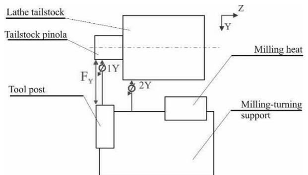
Fig. 3. Distribution of measuring points during the investigation of the quill (sensor 1Y) and tailstock (sensor 2Y) of the lathe TV 240 CNC
