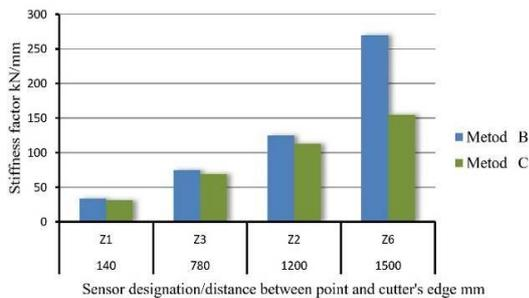
Fig. 9. Comparison of stiffness factors of the cutter in relation to the distance between measurement points and the cutter's edge
