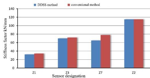
Fig. 10. Comparison of stiffness factors determined according to conventional method and DDSS method for the top position cutter of milling FS-550 CNC
