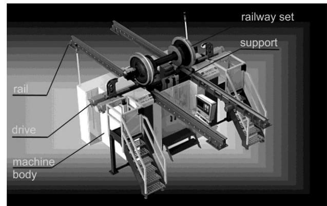
Fig. 11. Underfloor wheel lathe UGD 150 N [9]
