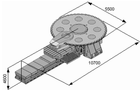
Fig. 6. Milling machine used for cranking FS-550 CNC CAD model with marked overall dimensions [8]
