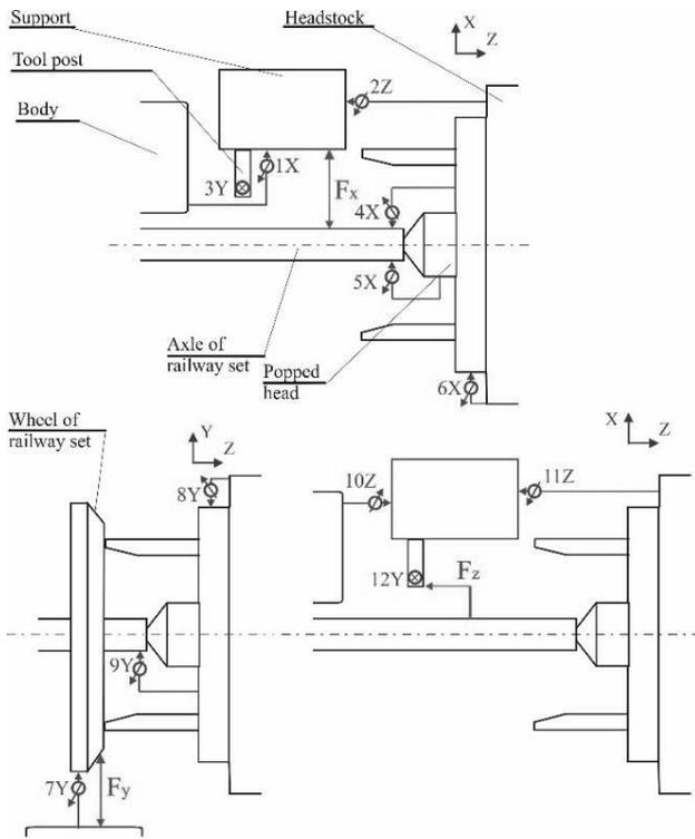
Fig. 12. Schemes of measurement systems during the investigation of circular mill UBF 112 N: a) for the forcing along X axle, b) for the forcing along Y
