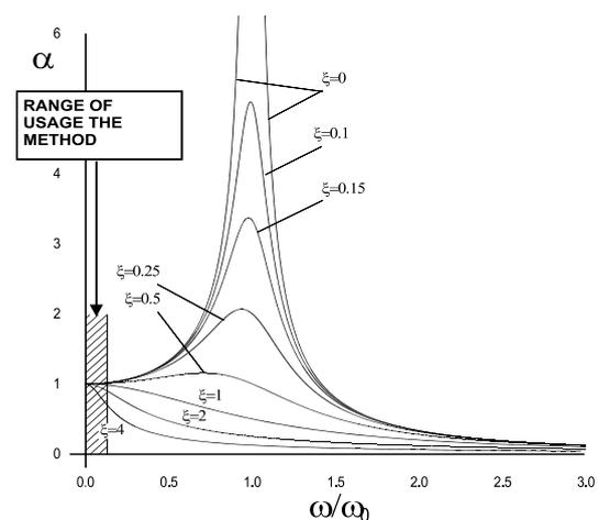
Fig.1. Graph of the multiplication index in the function of the relation of frequency of force exciting to frequencies of free vibrations;  $\omega_0$  - frequency of free vibrations [rad/s],  $\omega$  - frequency of the dynamic force [rad/s],  $\xi$  - dimensionless damping coefficient,  $\alpha$  - dimensionless multiplication index of the amplitude [7]
