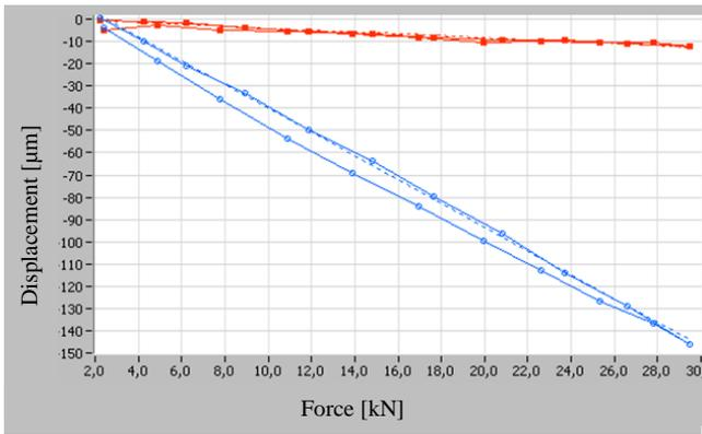
Fig. 4. Stiffness characteristics of the quill and the body of tailstock, as relative to lathe carriage: sensor 1Y – blue, sensor 2Y – red
