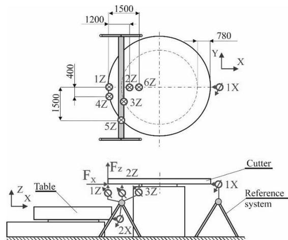
Fig. 7. Scheme of the measurement system used for investigation of a milling machine FS-550CNC
