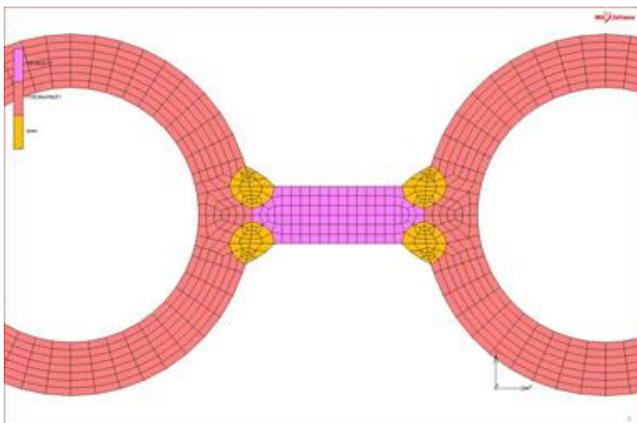
Fig. 3. Material distribution in the area of welded joint determined for the simulation purpose.
