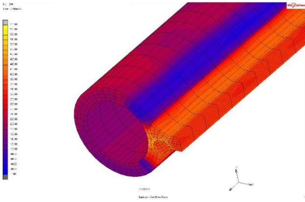
b. reduced stress after cooling to ambient temperature (before heat treatment)
