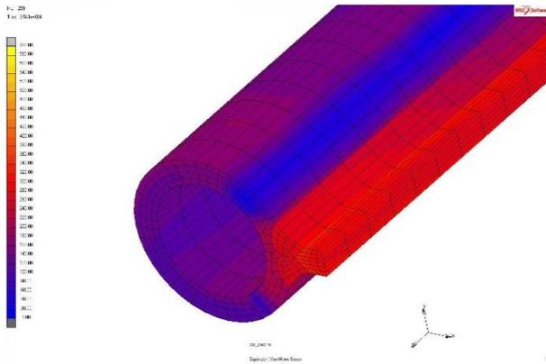
c. reduced stress after heat treatment and cooling to 300°C
