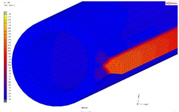
b. reduced displacements after cooling to ambient temperature (before heat treatment)
