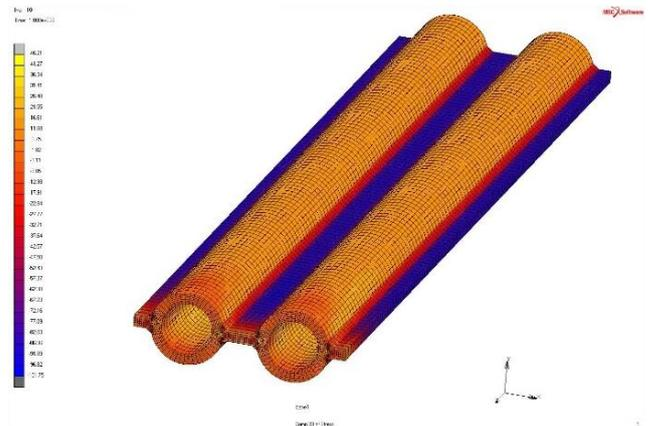
Fig. 7. Normal stress distribution ( $\sigma_z$ ) for SYM2 (MPa)
