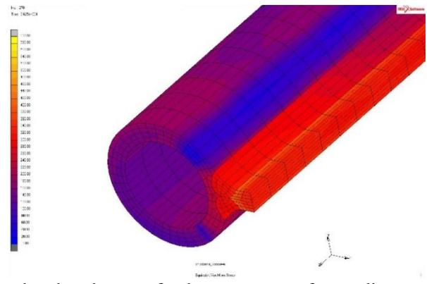
d. reduced stress after heat treatment after cooling to ambient temperature
