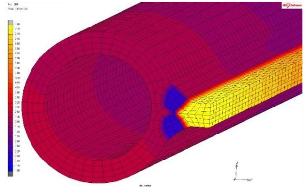
c. reduced displacements after heat treatment and cooling to 300°C
