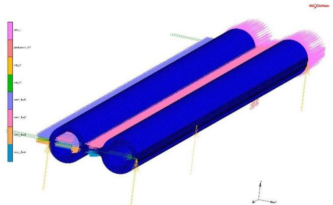
Fig. 5. Boundary conditions for complex case of the welding process.
