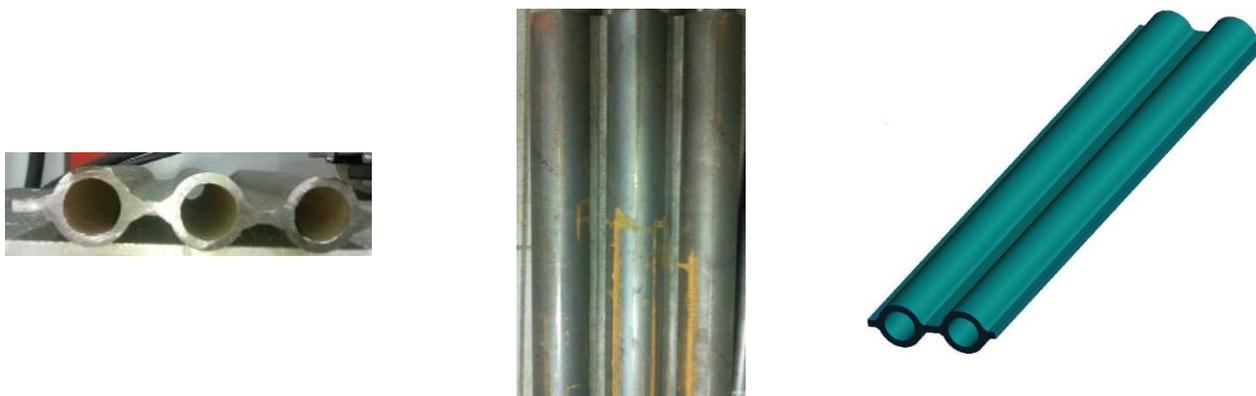
Fig. 1. Fragment of a membrane wall
