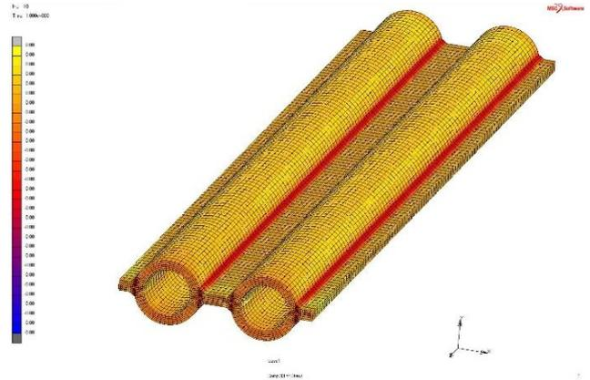
Fig. 6. Normal stress distribution ( $\sigma_z$ ) for SYM1 (MPa)
