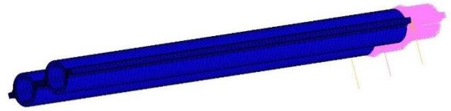
Fig. 4. Boundary conditions for a simple simulations of the influence of various types of material on state of stress and displacement
