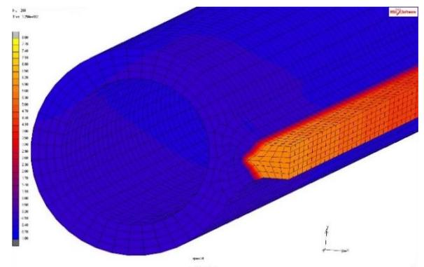
a. reduced displacements after welding
