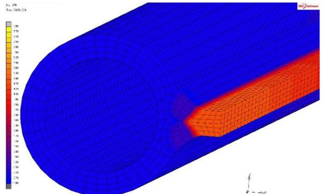
d. reduced displacements after cooling to ambient temperature
