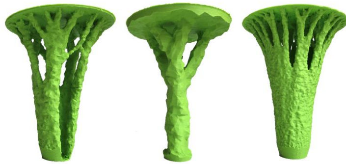
Fig. 1. Transition from a column to branch structures, [1]
