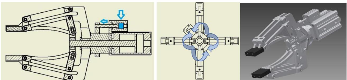
Fig. 3. The switch principle between 2 and 4 finger design
