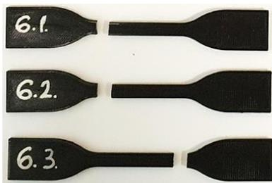
Fig. 16. Type 6 PLA specimens after tensile tests
