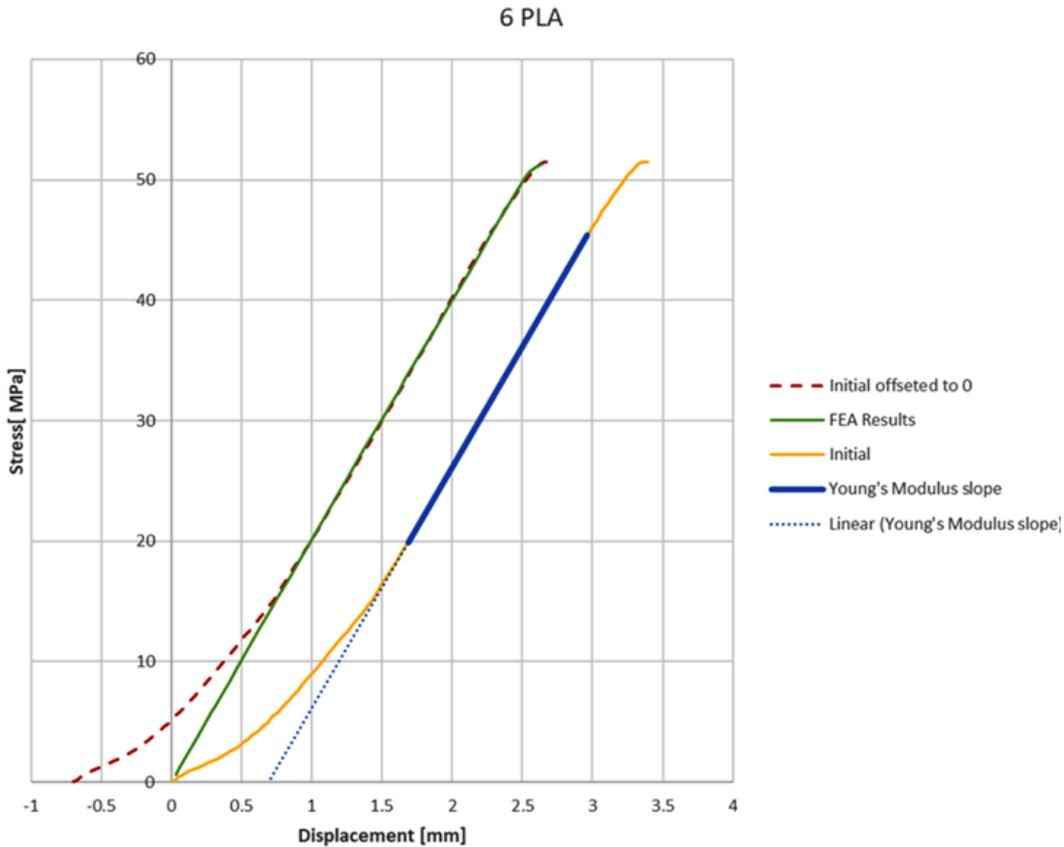
Fig. 13. Converting the stress-displacement curve, and the overlap of FEA with real test
