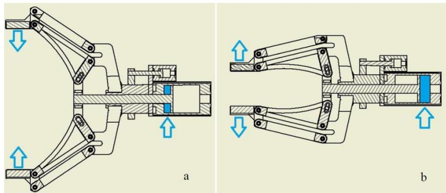
Fig. 2. Opening-closing principle using a pneumatic cylinder (a – closing; b – opening)
