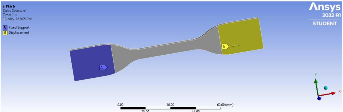
Fig. 14. Setup of the specimen on Ansys
