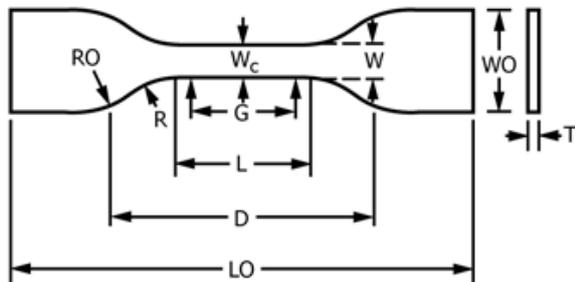
Fig. 5. Specimen geometry [6]
