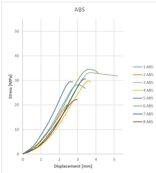
Fig. 12. Stress – displacement diagram for ABS specimens
