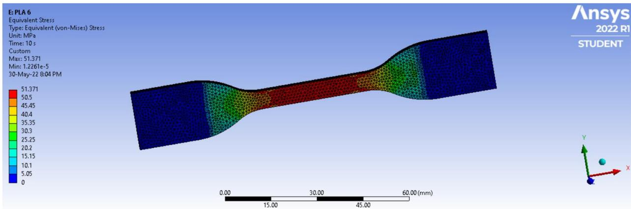
Fig. 15. FEA results on specimen (Ansys)
