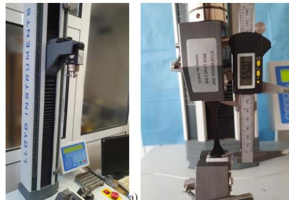
Fig. 10. Testing equipment (a – general view of machine; b – gripped specimen and the distance between grippers)
