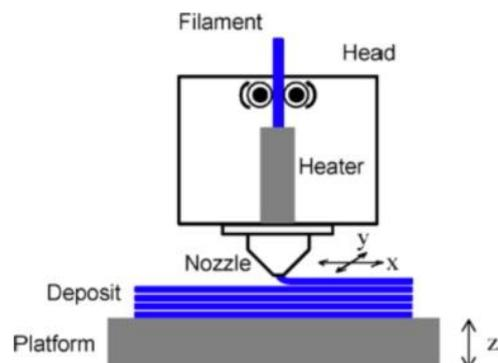
Fig. 4. A Schematic Diagram of FDM [7]
