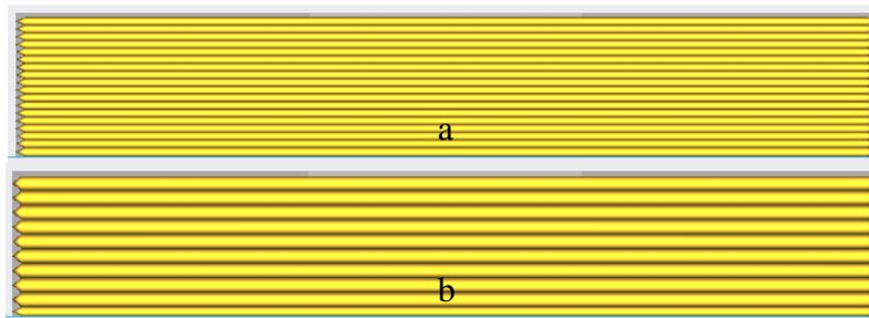
Fig. 8. Layers thickness (a – 0.17mm, b – 0.33mm)
