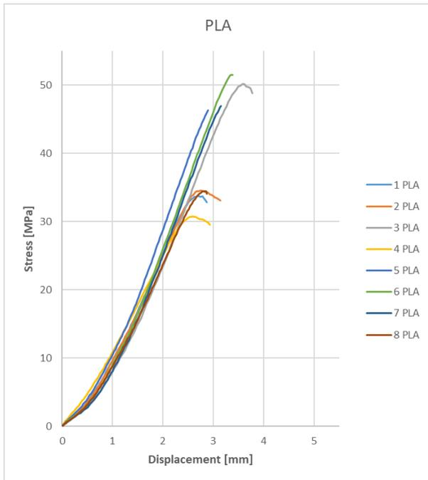
Fig. 11. Stress – displacement diagram for PLA specimens
