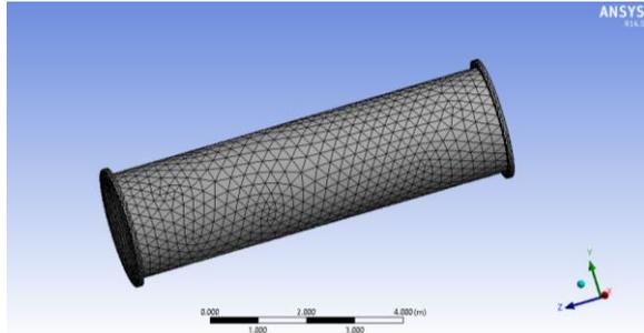
Fig. 3. The meshed design of propeller shaft
