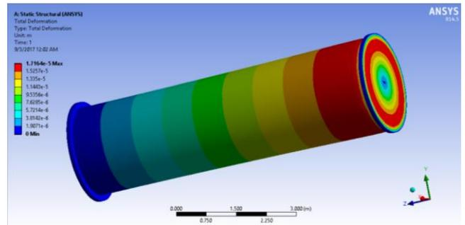
Fig. 5. Total deformation diagram – scenario 1
