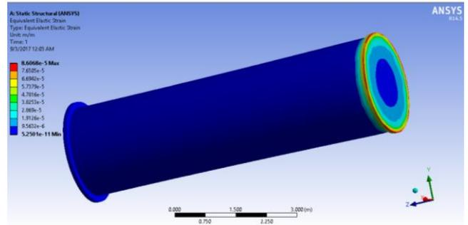
Fig. 6. Equivalent elastic strain-scenario 1
