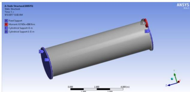
Fig. 4. Propeller shaft loading – scenario 1
