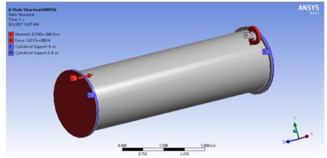
Fig. 12. Propeller shaft loading – scenario 3
