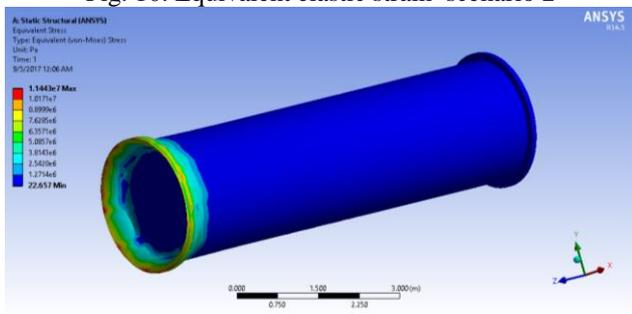
Fig. 11. Equivalent stress. – scenario 2
