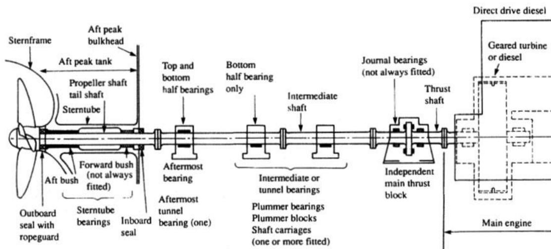
Fig. 1. Propeller shaft system [1]
