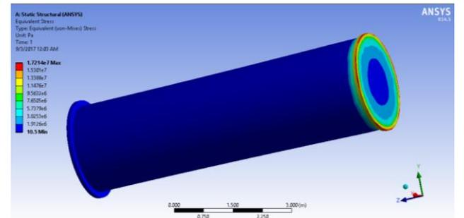
Fig. 7. Equivalent stress – scenario 1
