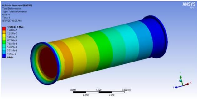
Fig. 9. Total deformation diagram – scenario 2
