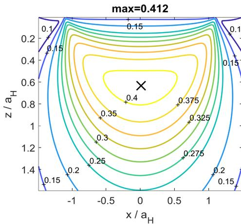
Fig. 2. Iso-contours of dimensionless equivalent von Mises stress due to pressure,  $\sigma_{VM}^p / p_H$ .
