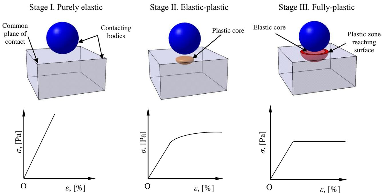
Fig.1. The stages in the plastic zone development and the schematic of the associated stress-strain ( $\sigma - \varepsilon$ ) relationship
