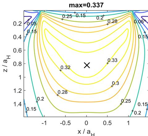
Fig. 4. Iso-contours of dimensionless total equivalent von Mises stress  $\sigma_{VM} / p_H$ .
