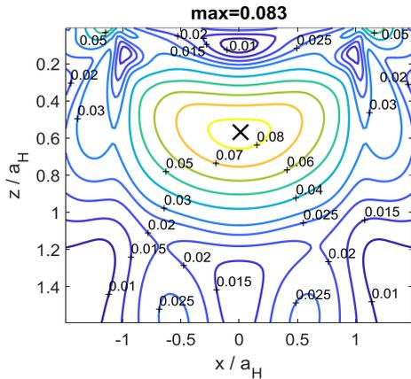
Fig. 3. Iso-contours of dimensionless equivalent von Mises stress due to plastic strains,  $\sigma_{VM}^r / p_H$ .
