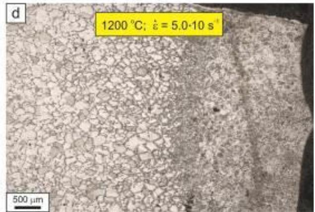
Fig. 14. Microstructures of samples after hot tensile test, revealed near the fracture area: a) and b) test temperature of 1050 °C and 1200 °C, strain rate of  $2.5 \cdot 10^{-3} \text{ s}^{-1}$  c) and d) test temperature of 1050 °C and 1200 °C; strain rate of  $5 \cdot 10^{-3} \text{ s}^{-1}$
