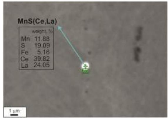
Fig. 13. The partially modified MnS-type inclusion in Fe-0.05C-24Mn-3.5Si-1.6Al steel
