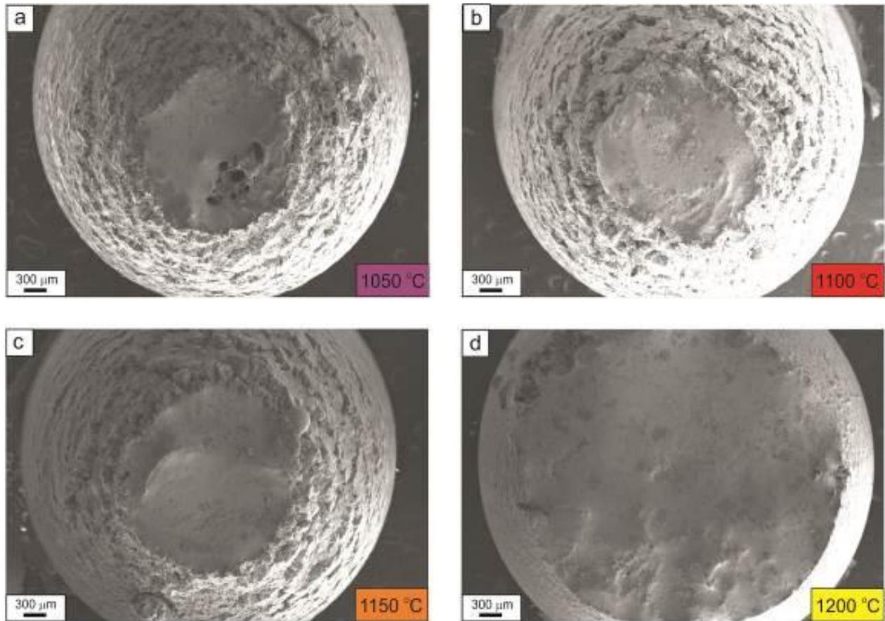
Fig. 9. Fractures of samples after tension at the temperature of: a) 1050 °C, b) 1100 °C, c) 1150 °C, d) 1200 °C (strain rate  $5 \cdot 10^{-3} \text{ s}^{-1}$ )
