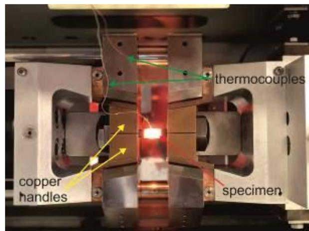
Fig. 3. Gleeble 3800 simulator chamber during high-temperature tensile test
