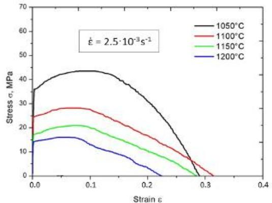
Fig. 5. Influence of plastic deformation temperature on a shape of  $\sigma$ - $\epsilon$  for the high-Mn steel (strain rate  $2.5 \cdot 10^{-3} \text{ s}^{-1}$ )
