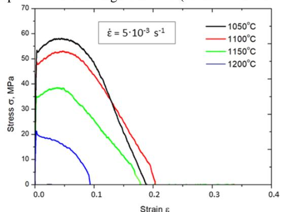
Fig. 6. Influence of plastic deformation temperature on a shape of  $\sigma$ - $\epsilon$  for the high-Mn steel (strain rate  $5 \cdot 10^{-3} \text{ s}^{-1}$ )
