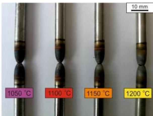
Fig. 8. View of the specimens after the hot tensile test (strain rate  $5 \cdot 10^{-3} \text{ s}^{-1}$ )
