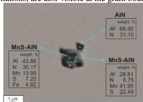
Fig. 11. Morphology and chemical composition of particles in Fe-0.05C-24Mn-3.5Si-1.6Al steel
