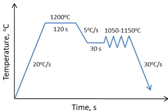
Fig. 4. Scheme of high-temperature tensile test
