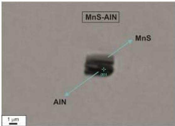
Fig. 12. View of the complex particle MnS-AlN-type in Fe-0.05C-24Mn-3.5Si-1.6Al steel
