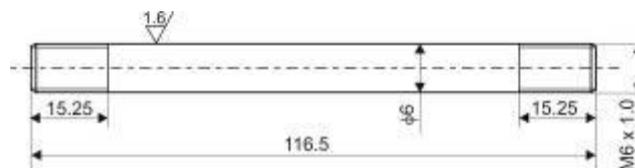
Fig. 2. Shape and dimensions of the sample used in high-temperature tensile test
