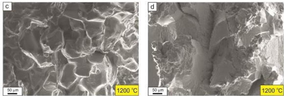
Fig. 10. Fractures of samples after hot tensile test: a, b) ductile fracture with numerous pits and voids of various size and depth, c) intercrystalline fracture; d) mixed fracture with visible cracks and flat grain surfaces (strain rate  $5 \cdot 10^{-3} \text{ s}^{-1}$ )
