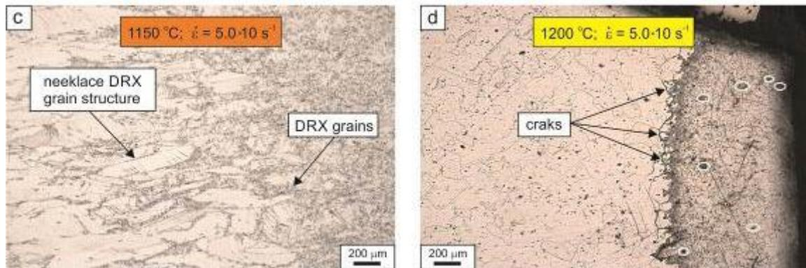
Fig. 15. Microstructure of samples after hot tensile test: a) and b) at the temperature of 1050 °C; c) at the temperature of 1150 °C; d) at the temperature of 1200 °C; (strain rate  $5 \cdot 10^{-3} \text{ s}^{-1}$ )
