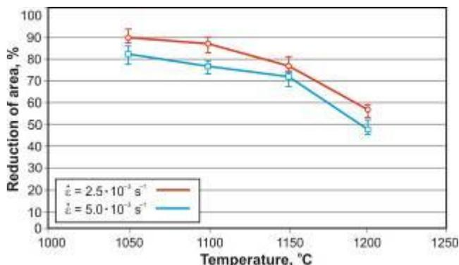
Fig. 7. An influence of plastic deformation temperature and strain rate on the changes of reduction of area
