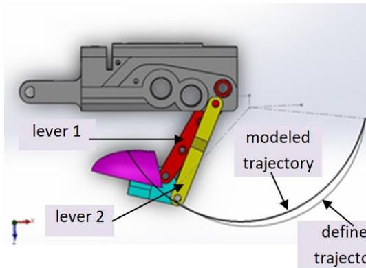
a. first iteration, different defined and modeled trajectories
