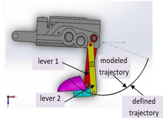
b. final iteration, identical defined and modeled trajectories
