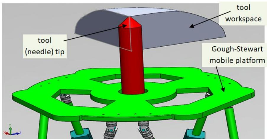
Fig. 2. 3D Workspace generated with Solidworks-API.
