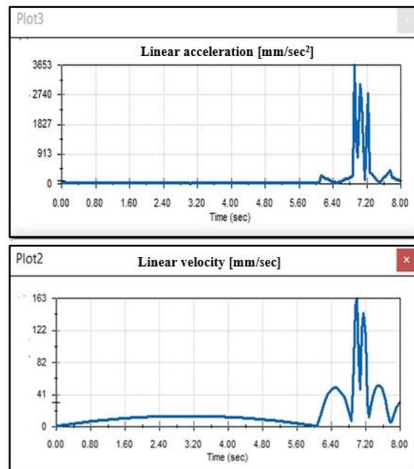
Fig. 6. Linear acceleration magnitude during movement measured at tools location using method B for optimization – final step.
