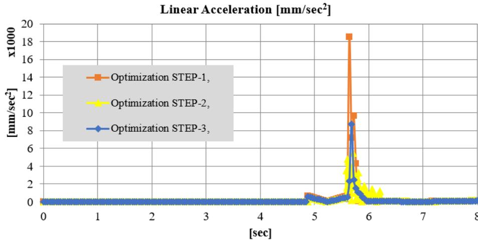
Fig. 5. Linear acceleration magnitude during movement measured at tools location using method, A for optimization.
