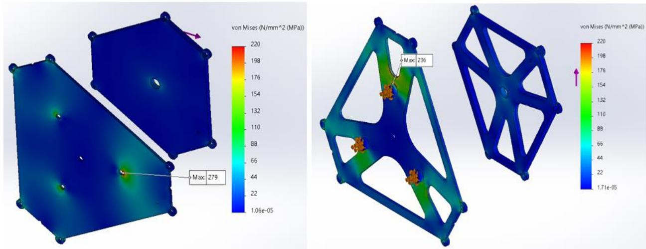
Fig. 7. Topologic optimization from the initial model (left) to the design from right side based on multiple criteria: weight, material, maximum stress.
