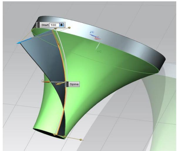
Fig. 7. “Curve surface” (orange) and “Law extension” operations
