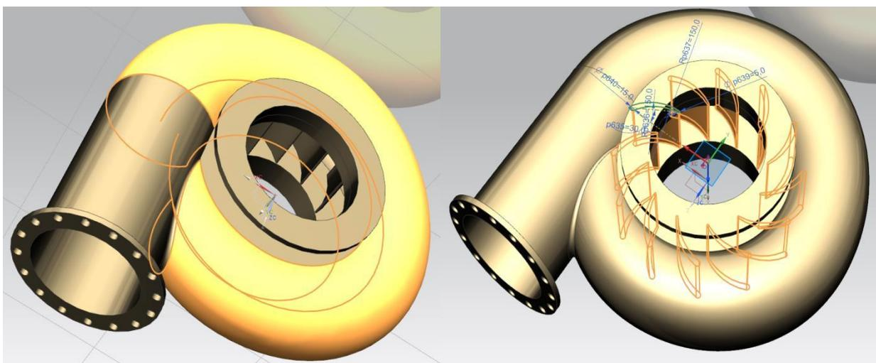
Fig. 5. Spiral turbine casing with spline guide curve, swept operation (orange) and stator blades
