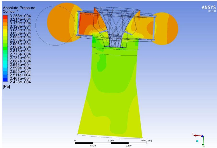
Fig. 12. Absolute pressure – vertical section field
