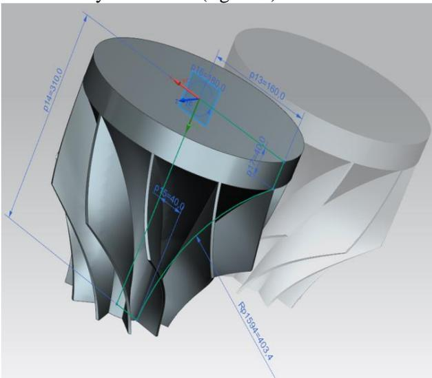
Fig. 6. “Revolve” of sketch (green) and dimensions
