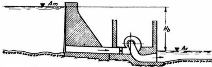
Fig. 2. Upstream water storage ( $A_m$ ) and the downstream water drainage channel ( $A_v$ ) at hydropower plant with turbine [1]
