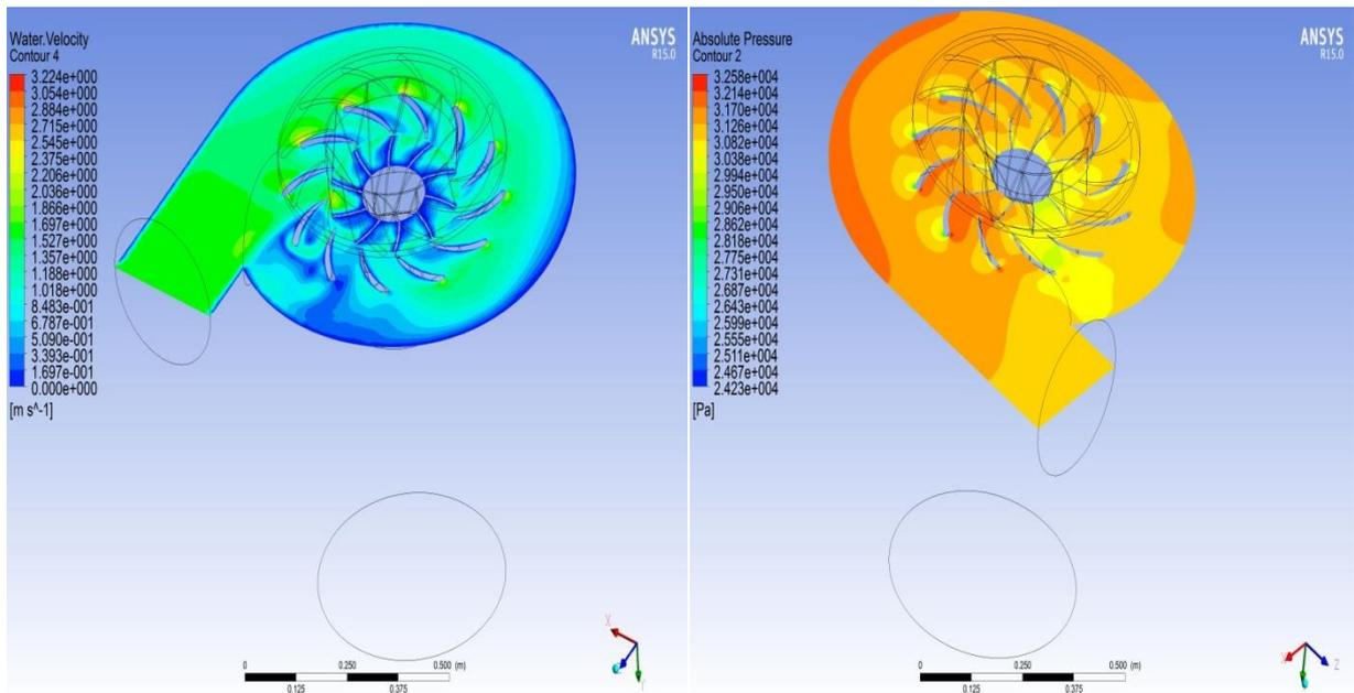
Fig. 13. Velocity and absolute pressure – orizontal section fields
