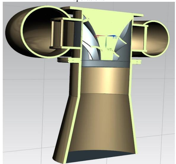
Fig. 8. Assembled NX CAD models (section viewing), spiral casing, impeller and diffuser
