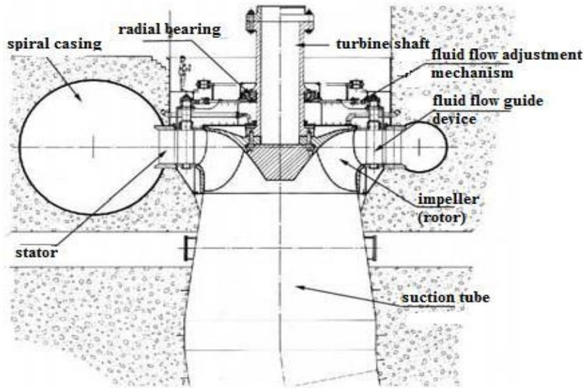
Fig. 1. Francis turbine component parts – axial section, [1]
