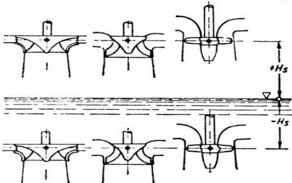
Fig. 4. The middle plane of the fluid flow guide device at the Francis turbine [1]
