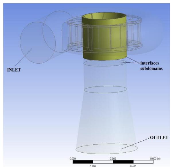
Fig. 9. Impeller subdomain (the rotating one) surrounded by two other static fluid subdomains, (one is coloured in green the other is transparent)
