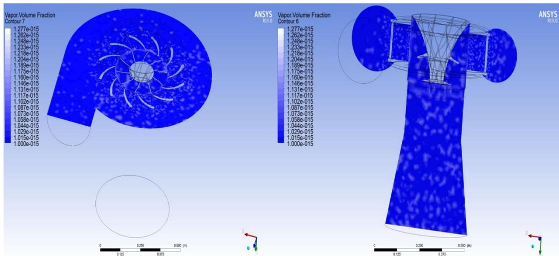
Fig. 14. Vapour Volume Fraction – horizontal and vertical section fields
