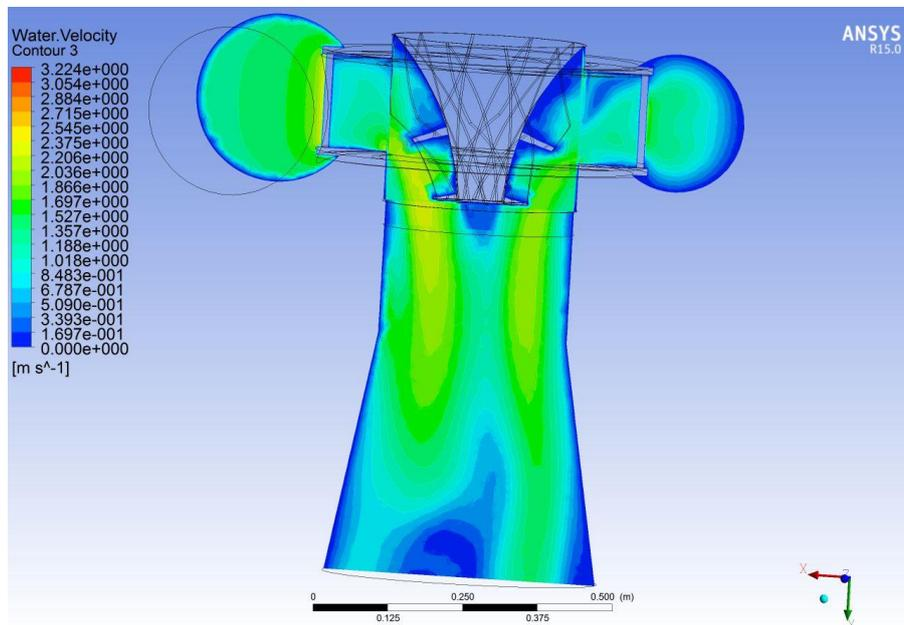
Fig. 11. Water velocity – vertical section field
