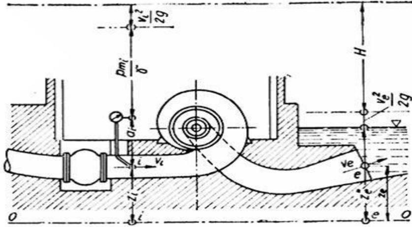
Fig. 3. Input and output parameters for the Francis turbine [1]
