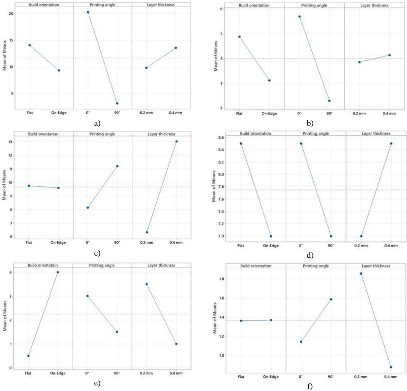
Fig. 2. Main effect plots for a) tensile strength, b) tensile modulus, c) surface roughness, d) material usage, e) scrap material, f) energy consumption
