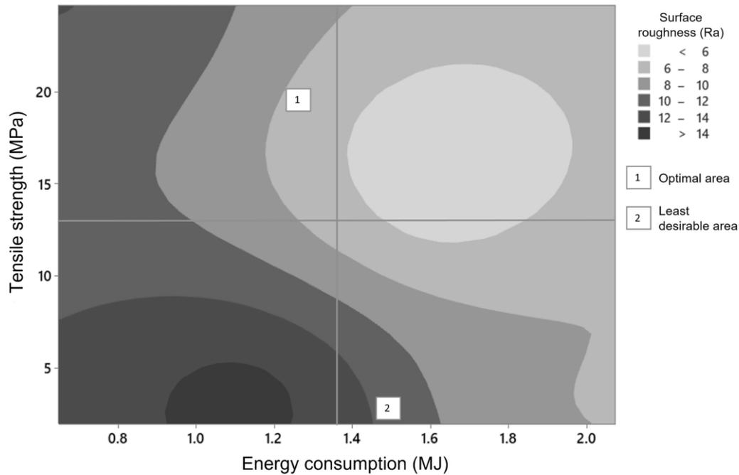
Fig. 3. Contour plot of tensile strength versus energy consumption versus surface roughness
