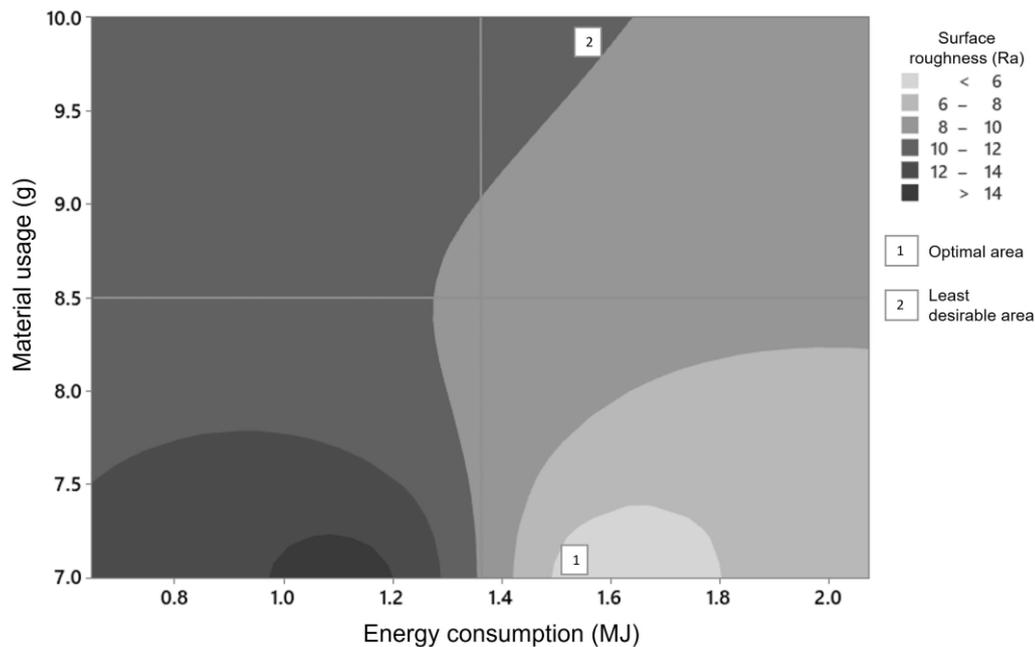
Fig. 4. Contour plot of material usage versus energy consumption versus surface roughness
