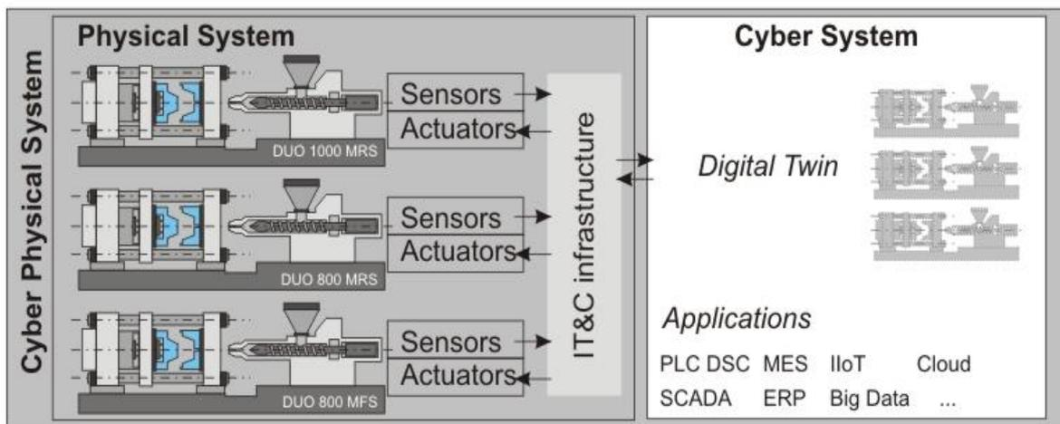
Fig. 2. The architecture of the Cyber Physical System
