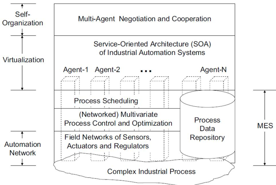
Fig. 1. New framework of re-configurable industrial automation [5]
