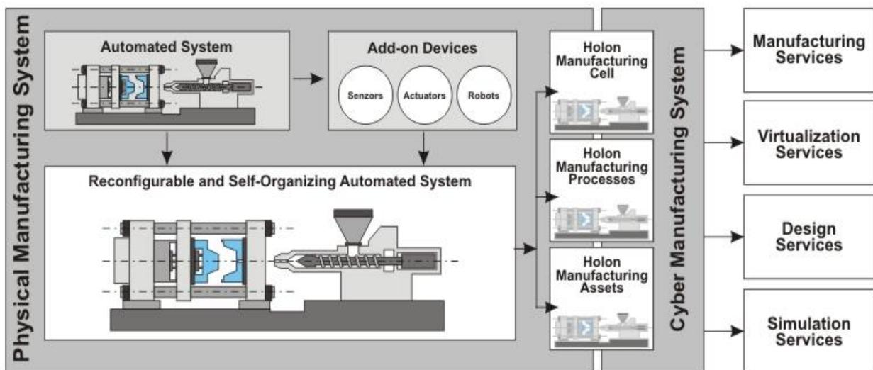
Fig. 3. Defining Holons in Industry 4.0 Manufacturing System
