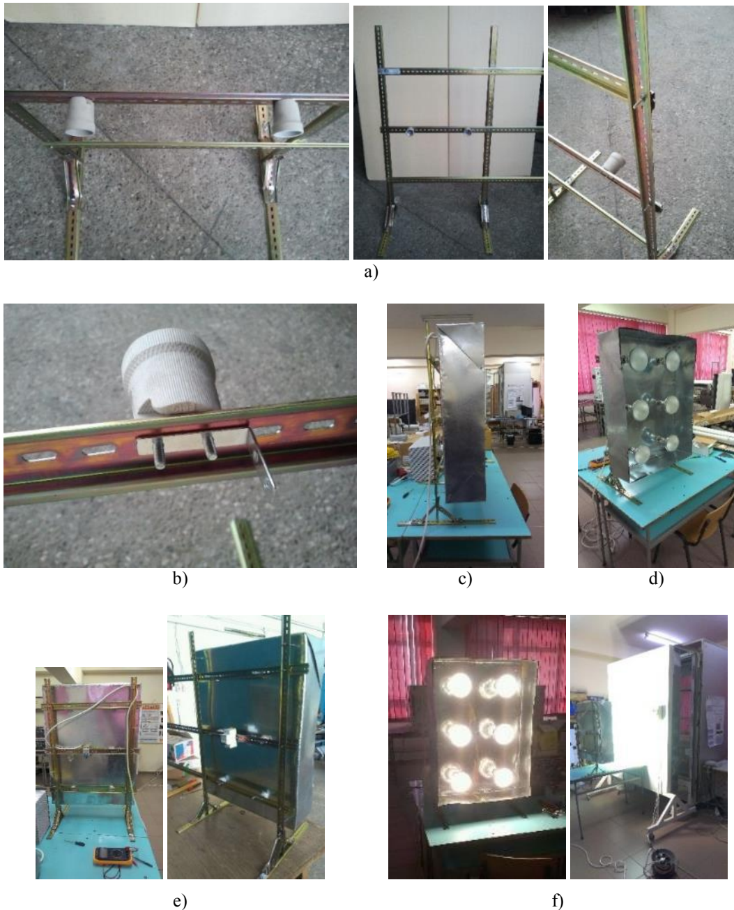
Fig. 10. Execution steps (a - support frame, b - E27 socket; c - reflective plate positioning, d - light source mounting, e - electrical connections, f - functional testing)
