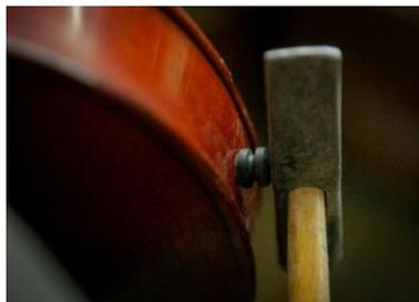
(s) Inserting the end pin
