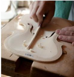
(g) Attaching the resonance bar
