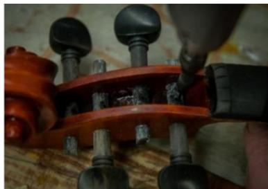
(t) Inserting and drilling the pegs
