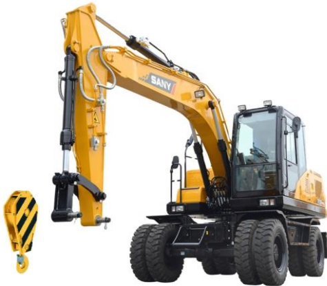
Fig. 3 Tire excavator with crane equipment, [1]
