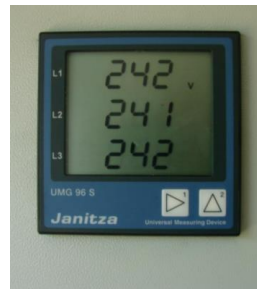
Fig. 2. Janitza system for real-time data retrieval and storage, [1]
