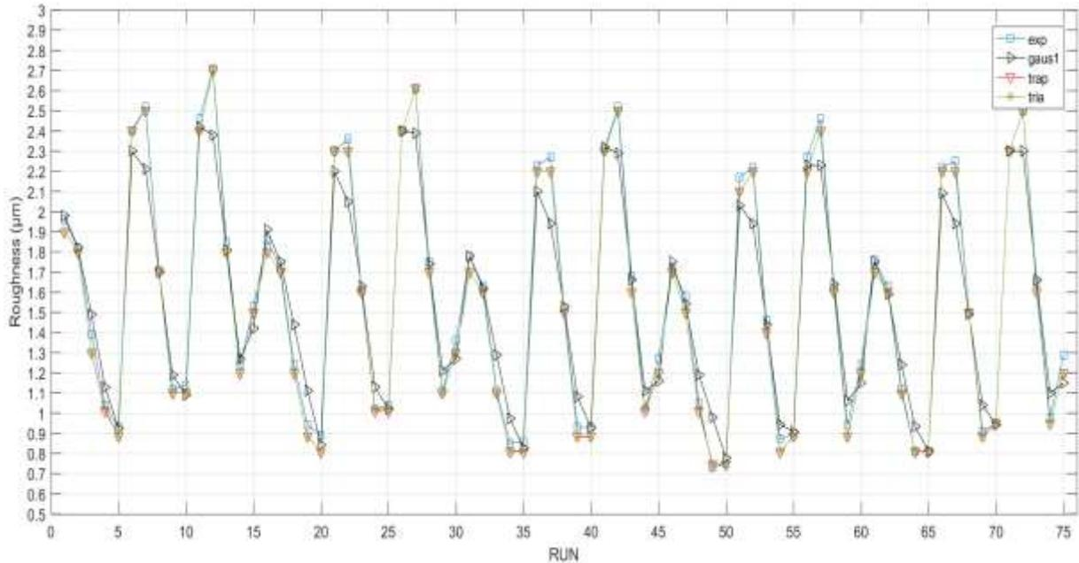
Fig. 10. Variation of roughness (Experimental, Trapezoidal, Triangular and Gaussian) according to the number of tests
