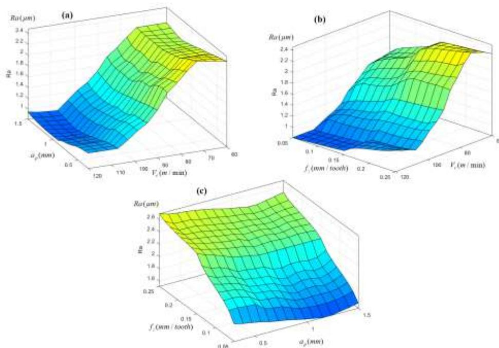
Fig. 11. Variation of the predicted roughness with the fuzzy logic model as a function of the cutting parameters
