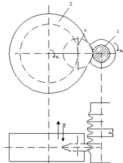
Fig. 1. Kinematics of the process with one roller
