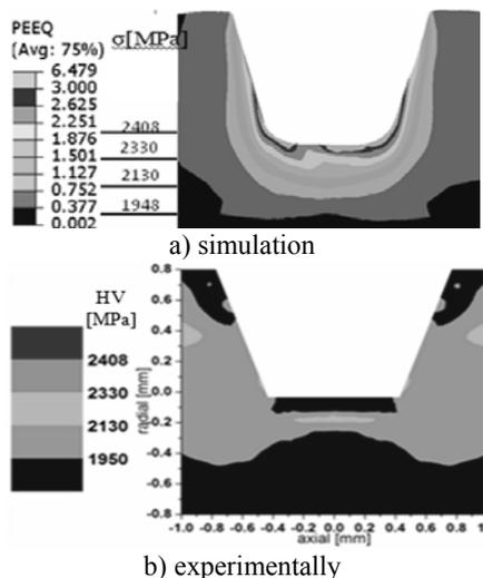
Fig. 10. Distributions of equivalent deformations obtained through simulation and experimentally for sample 2
