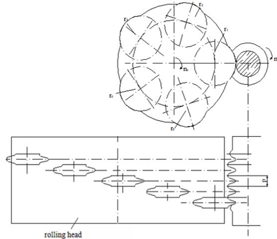
Fig. 2. Kinematics of the process with several rollers
