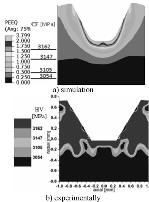
Fig. 12. Distributions of equivalent deformations obtained through simulation and experimentally for sample 4
