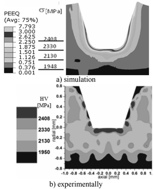
Fig. 11. Distributions of equivalent deformations obtained through simulation and experimentally for sample 3
