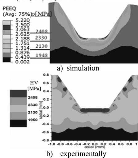
Fig. 9. Distributions of equivalent deformations obtained through simulation and experimentally for sample 1
