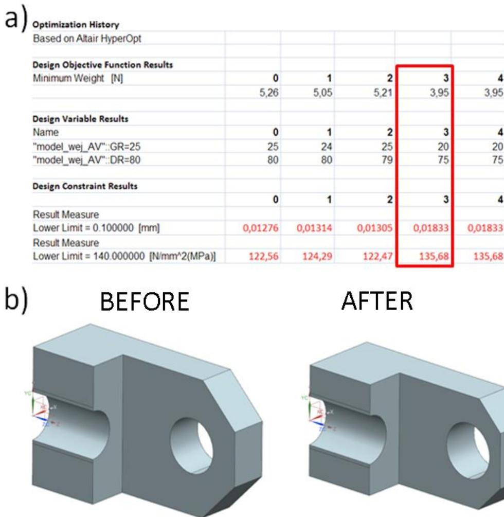
Fig. 7. Results of parametric optimization (in NX Geometry Optimization module):
