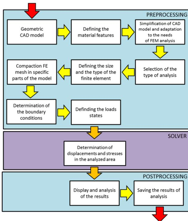
Fig. 1. Stages of the FEM-based structural analysis
