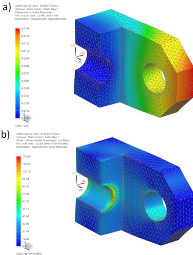
Fig. 3. Results of the FEM-based structural analysis:
