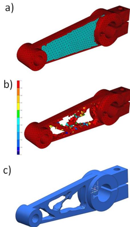
Fig. 5. Selected stages of the topology optimization process (in TOSCA STRUCTURE software):
