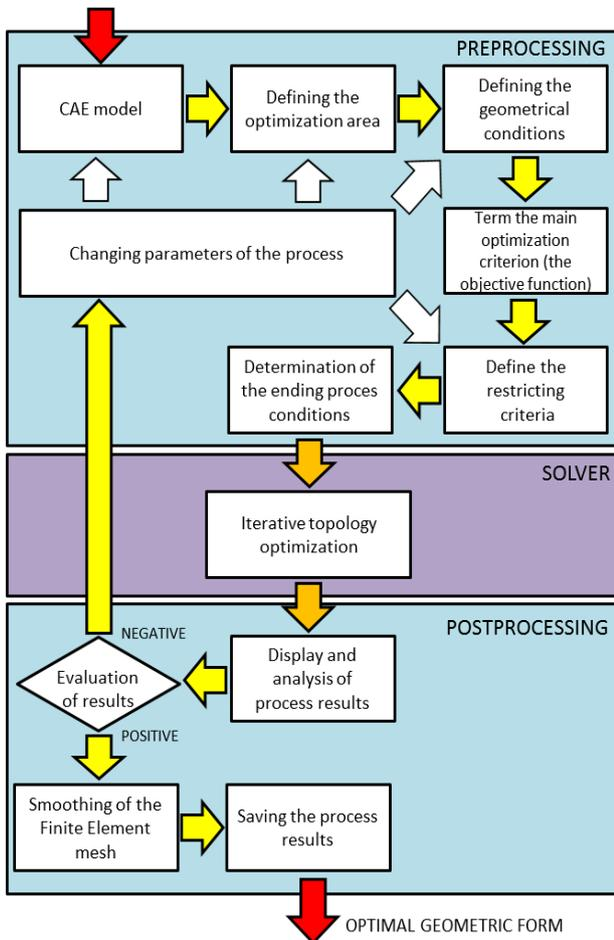
Fig. 4. Stages of the geometric form optimization process
