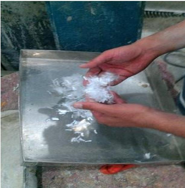
Fig.1. Woolen Polypropylene (WPP) fiber
