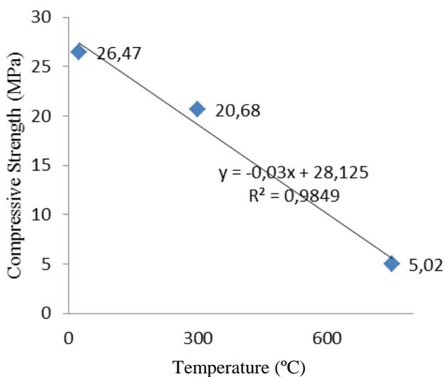
Fig.4. Compressive strength of 600 g WPP specimens
