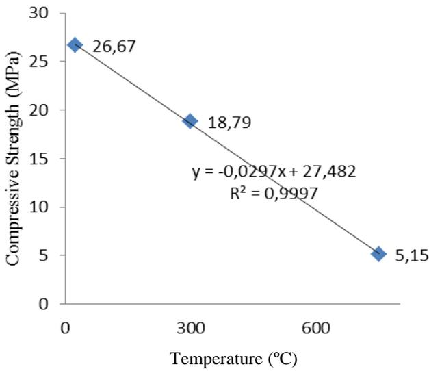
Fig.2. Compressive strength of control specimens
