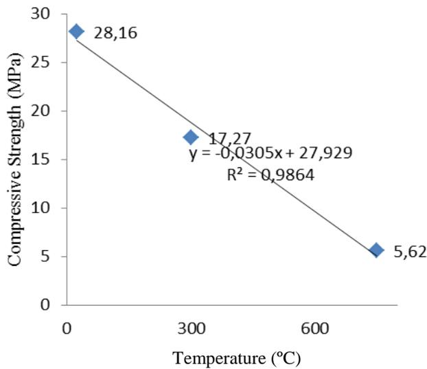
Fig.3. Compressive strength of 300 g WPP specimens
