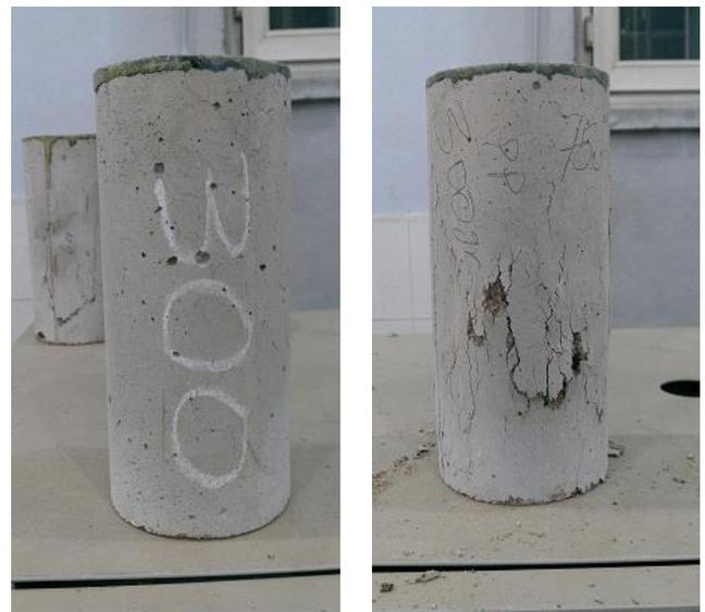
Fig.6. Fiber reinforced concrete (300g WPP) specimens before and after being exposed to 750°C
