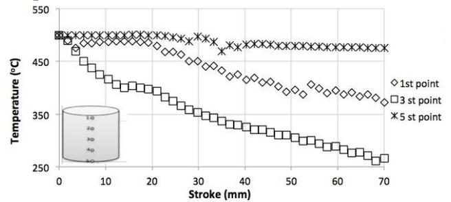
Fig 6. Temperature variations occurring at point nos. 1, 3, 5 on the billet in the unheated container
