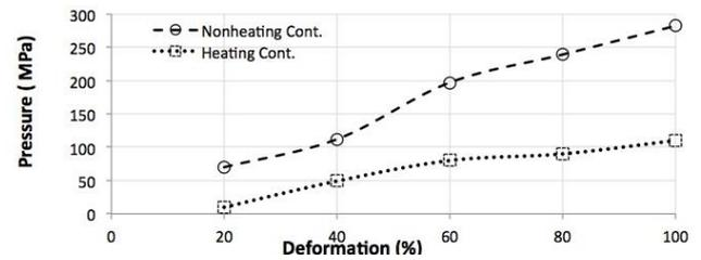
Fig 8. Variation of extrusion pressure in heated and unheated containers
