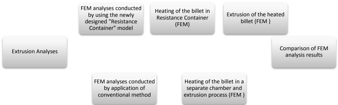
Fig 3. Flow Chart of FEM Analyses
