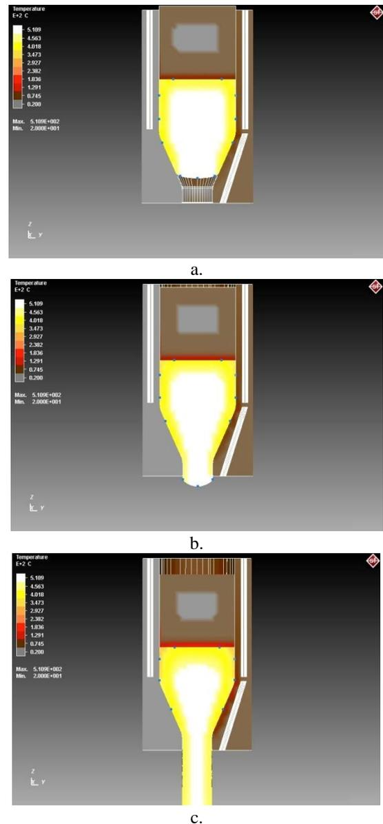
Fig 4. Temperature variations occurring in the billet during the extrusion process (unheated container)
