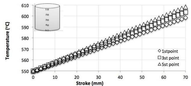
Fig 7. Temperature variations occurring at point nos.1, 3, 5 on the billet in the heated container
