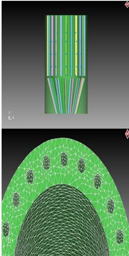
Fig 1. Location of the points on workpiece (a) and meshing (b)
