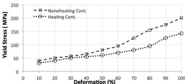
Fig 9. Stress values developing in the billet according to conventional and new container designs
