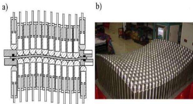
Fig. 2. Reconfigurable surface tooling:(a) multi-punch stamping die; (b) multipoint forming press machine YAM8-315, [12]
