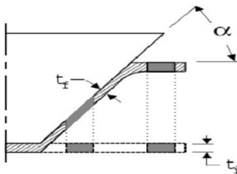
Fig.5. Deformation of an element in a shear formed cone, [8]
