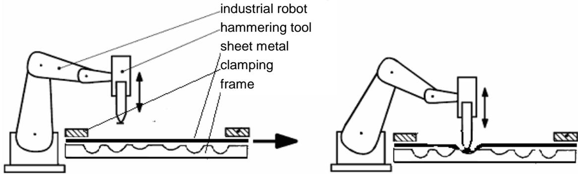
Fig. 1. Principle of the incremental hammering by an industrial robot, [6]
