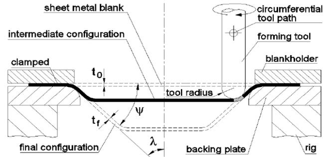
Fig. 6. Schematic representation of a cross section view of SPIF process, [8]
