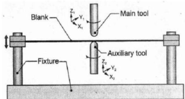
Fig. 7. Schematic representation of Incremental Forming with Counter Tool, [8]
