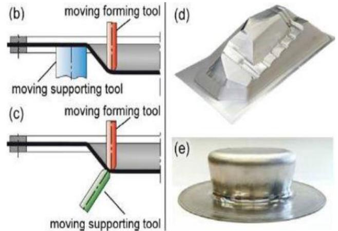
Fig.11. (a) Roboforming setup, (b) P-DPIF, (c) L-DPIF, (d) Complex automobile part, (e) A part with negative wall angle ( $-7^\circ$ ), [1]
